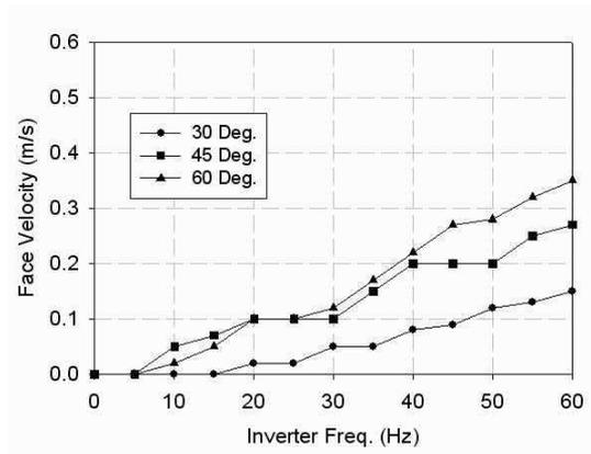
Fig. 9 Face Velocity with VVVF inverter frequency
