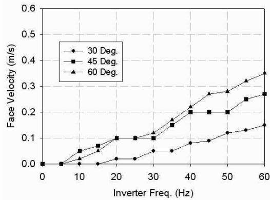
Fig. 9 Face Velocity with VVVF inverter frequency
